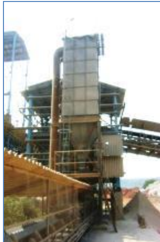
Bag filters at various material transfer points & silo top
