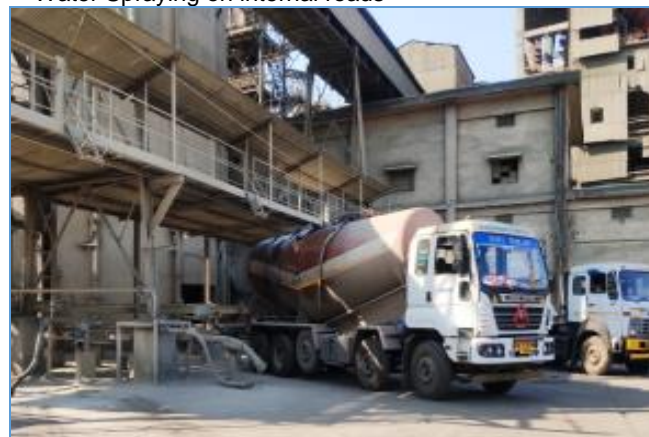
Pneumatic handling of Flyash
