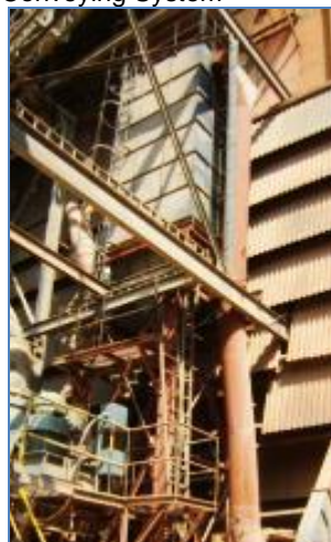
Bag filters at various material transfer points & silo top
