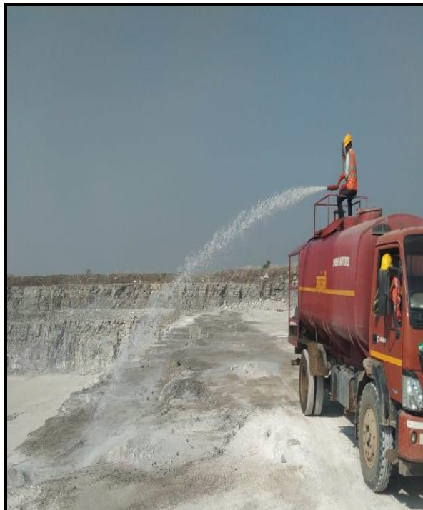
Water sprinkling on drill hole face before blasting and water sprinkling for dust suppression on blasted muck pile
