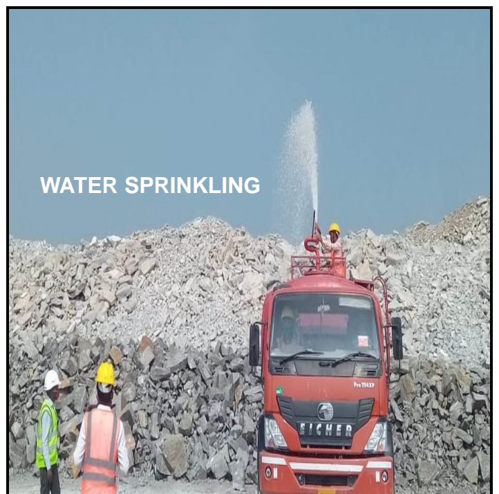
Water sprinkling on drill hole face before blasting and water sprinkling for dust suppression on blasted muck pile
