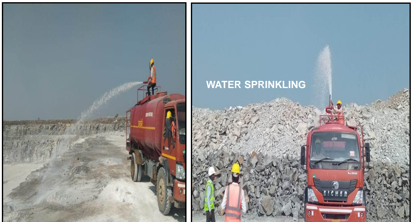
Water sprinkling on drill hole face before blasting and water sprinkling for dust suppression on blasted muck pile
