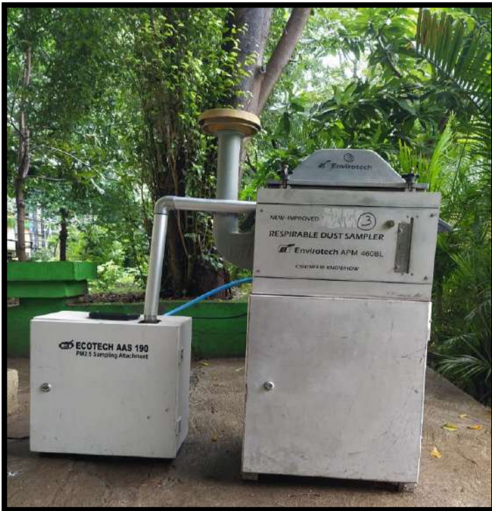
RDS Sampler & Stack Monitoring Kit Available for In-house Ambient Air Monitoring as well as Stack Monitoring
