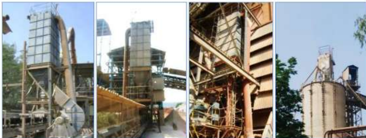
Bag filters at various material transfer points & silo top
